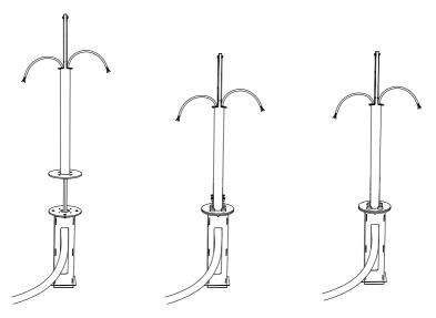
Make sure the pedestal bracket is facing the way you want it to. When properly positioned, fix the pedestal to the anchor slot with 3 screws.
