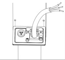
2) Use the provided 2 M5x16 screws (Torque 1.2Nm) to secure the cable block onto the bottom of the pedestal bracket.
